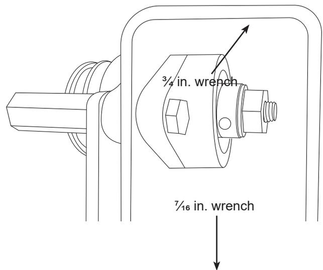
8. Ensure tension is set correctly on the X chain and cable combination. Locate the adjustment turnbuckle. Using a  $\frac{7}{16}$  in. wrench, loosen the adjustment turnbuckle until it can be turned by hand, without using the wrench. To set tension, tighten the turnbuckle by hand as much as possible. Once the turnbuckle cannot be turned by hand, tighten it one full rotation using a  $\frac{7}{16}$  in. wrench. Tension for the X chain is now set.
