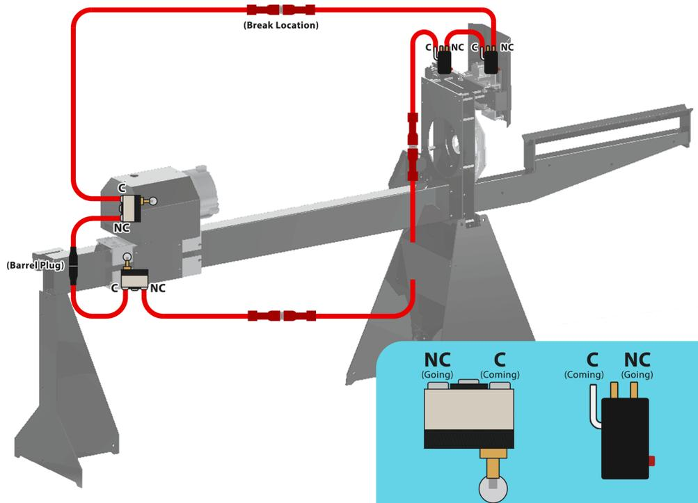
It is possible to bypass a limit switch on the A150 by rerouting the limit switch wiring to eliminate a limit switch. Unplug a limit switch from the loop and connect the wires from the limit switches on either side of that switch to “shorten” the loop. Refer to the diagram for reference.
