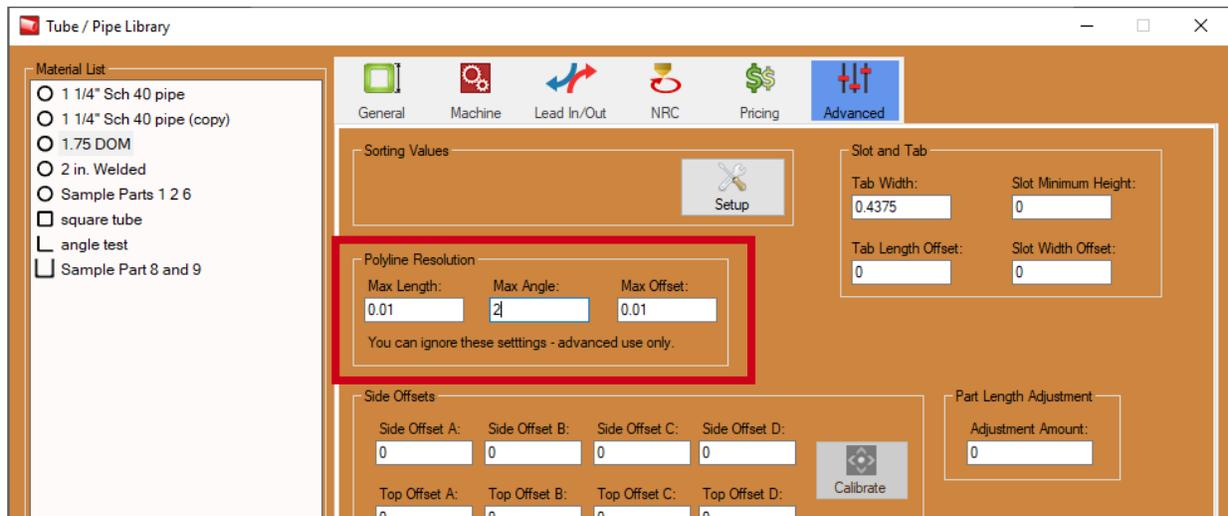
A final way to adjust cut rotation on the Dragon A150 machine involves editing Polyline Resolution in the Advanced option in the Tube Library. While Bend-Tech does not recommend changing default Polyline Resolution settings, changing the settings slightly can result in more accurate cut rotation on the A150 machine.
