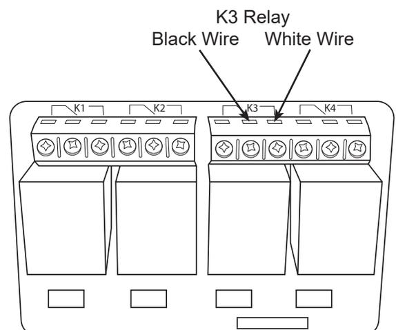
6. With the Torch wires secure in the relay, reassemble the Control Box. Reattach the Control Box cover plate.
