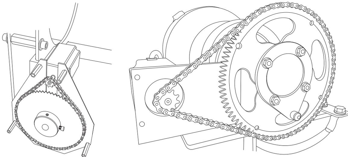
2. Using a  $\frac{5}{16}$  in. Allen wrench, remove the X Chain Cable Cover by removing the two screws.
