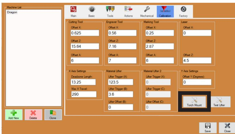
Click Torch Mount at the bottom right of the calibration screen. This will open the Torch Mounting Utility interface.
