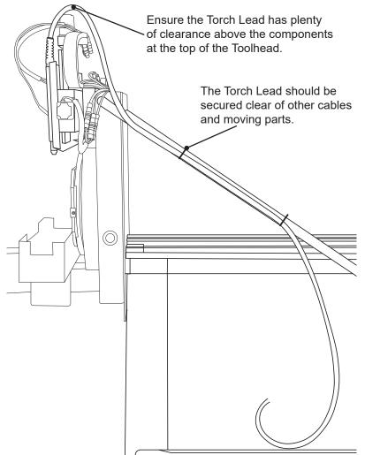
The Customer should ensure the Torch lead is secured so it is clear of the cables at the top of the Toolhead. It is recommended that the Torch lead be secured so it loops up above the components at the top of the Toolhead.
