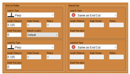
The operator can set the Lead In/Out for the material. Click Lead In/Out at the top of the interface.
