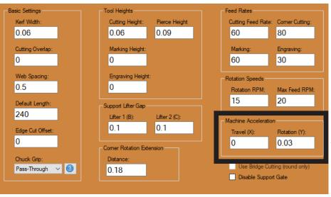
To set Y-Axis acceleration, on the Bend-Tech Dragon home interface, under Library, click Tube Library, then click the Machine icon. In the bottom right, in the Machine Acceleration box, change the Rotation (Y) value to .030 in.
