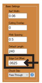
Under the Machine tab, in the Basic Settings box, set Edge Cut Offset to .0625. Edge Cut Offset is the distance beyond the edge of the material the Lead In/Out is allowed to extend when performing edge cuts. Bend-Tech has found .0625 to be the optimal setting when processing angle or channel material.
