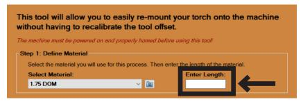
Enter the length of the material that will be loaded into the machine. Bend-Tech recommends using a piece of material 3-6 ft. in length to avoid material sagging.
