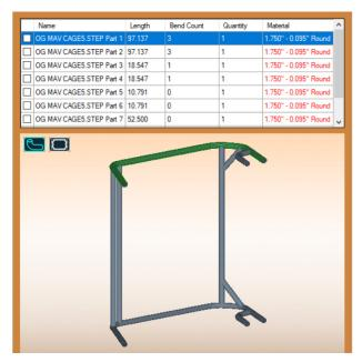
The Project Interface will feature a parts listing and a diagram of the assembly. The Operator can toggle between a diagram of the assembly and a flat layout by clicking the bent tube icon or the flat part icon in the top left corner.
