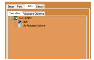
The Shifts tab will display the order of operation the machine will use for its cutting path. The Operator can use the Shifts feature to rearrange cutting actions, unassign or remove actions from the list.
