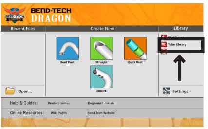
Before performing any type of cutting on the Dragon A400, the material being cut needs to be added the Tube and Pipe Library.
