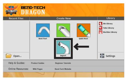
There are two ways to import a file into Dragon CAM. For the first method, click Import from the Dragon CAM task menu interface under Create New.
