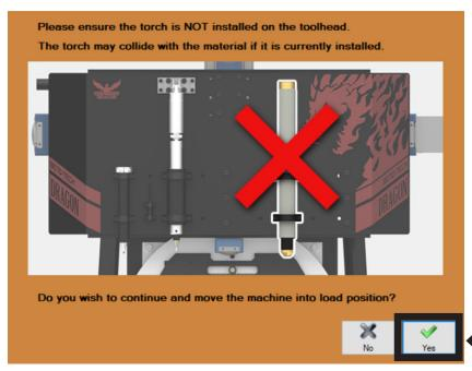
A Torch Collision Warning interface will appear. Check to confirm the Torch is raised enough that it will not contact the material before it can be adjusted. If the Torch is too low, adjust it so it is clear of the material.
