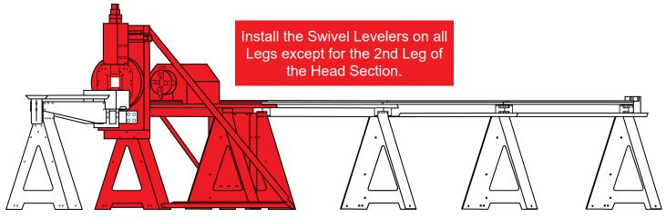
Install the remaining Swivel Levelers on leg #4, the un-numbered leg, and the two legs that make up the tail section of the machine.
