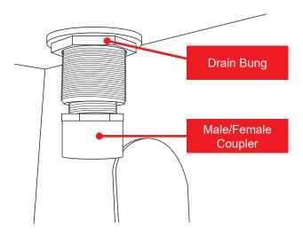
Also thread one PVC coupler into the bung inside the parts catcher. This will allow the parts catcher to hold water to help cool parts.
