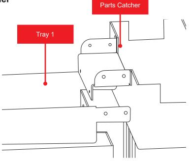
Use one of the support legs to support the free end of the Water Tray. Use four ¾ in. button head screws, nuts and washers to attach the side tabs on the coolant tray to the parts catcher. Feed the screws through the side of the coolant tray so the head of the screw is inside the coolant tray and the nut and washer are on the outside.
