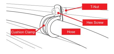
Locate the T-nuts and  $\frac{1}{2}$  in. hex screws from the hardware bag, along with the cushion clamps. Loop the cushion clamps around the hose, spacing evenly at intervals along the beam. Attach the cushion clamps to the beam using the T-nuts and hex screws.
