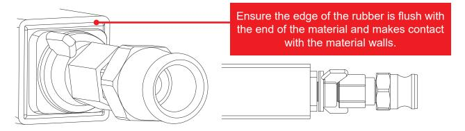
Tighten the Wing Nut until the plug is making contact on every side of the material walls. Seat the plug by tightening the Wing Nut five full turns to expand the plug into the material walls.
