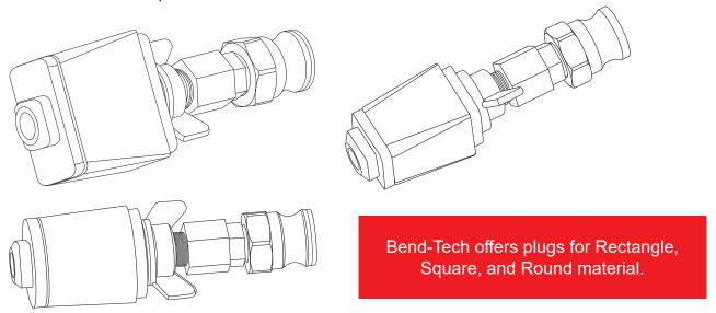
Insert the plug into the end of the material until the edge of the rubber is flush with the end of the material.
