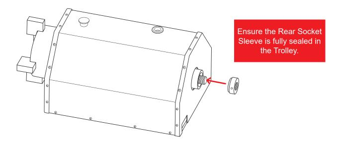
Thread the rear swivel assembly into place, do not over tighten.
