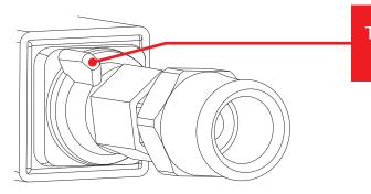
Tighten the wing nut five turns to expand the plug into the material walls.
