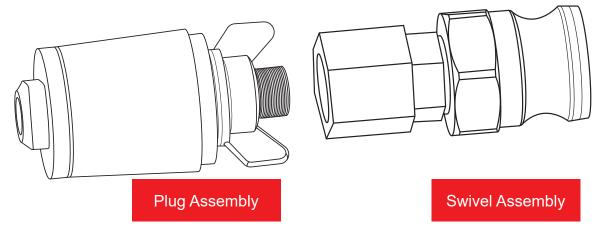
Screw the Swivel Assembly onto the Plug Assembly until a slight resistance is encountered.
